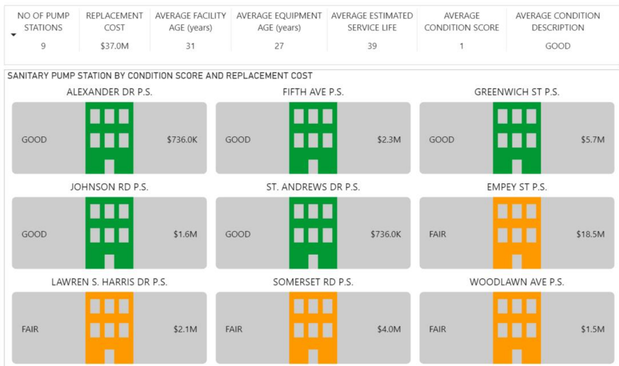
Figure 16: Wastewater Pump Station Asset Summary
